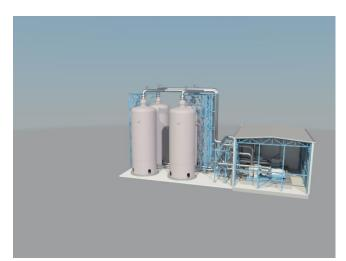
The GridScale energy storage consists of one or more sets of steel tanks filled with crushed stone. Charging and discharging is done with a system of compressors and turbines. The number of tank sets with stone filling can be varied, depending on the desired storage duration.
