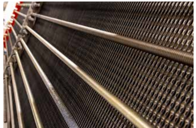
Novel electrode stack design: The electrode stack system of the HydroGen Electrolyzer is of a novel design that integrates cooling and reduces losses. The low-cost stack arrangement is designed for industrial-scale mass production.
