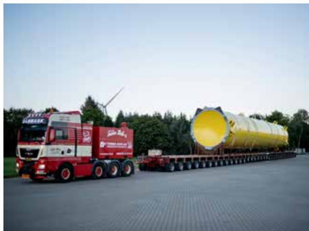
Road transport: Tetra components are suitable for road transport. Here, the TetraSpar center column is leaving Welcon's factory, heading for the port assembly site.
