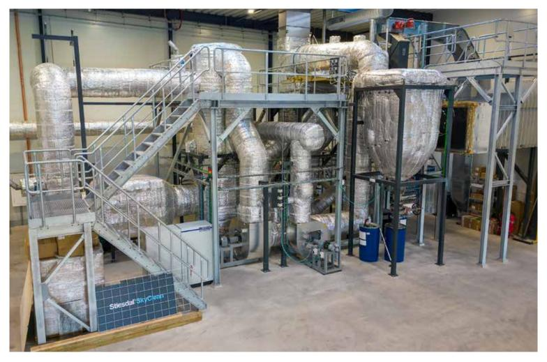
**Fully automated pyrolysis production:** Stiesdal SkyClean has developed a fully automated process plant capable of transforming almost any kind of biogenic feedstock into biochar and biofuels. The above image is from the 2 MW SkyClean plant in GreenLab, Skive.
