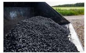
Biochar value stream: SkyClean pyrolysis produces high-grade, tar-free biochar suitable for spreading on farmland. Once stored in the soil, SkyClean biochar is a tradeable stable carbon sink.
