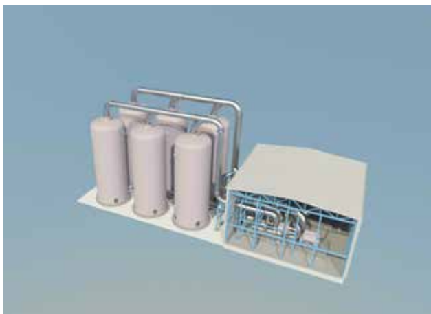
The basic design of GridScale: A single power unit and multiple pairs of hot and cold storage tanks.
